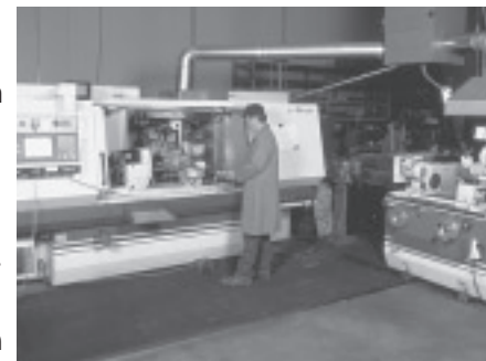
The CNC grinding cell has reduced set-up time by 60% and increased thru' put by 20% while holding more constant tolerances.
