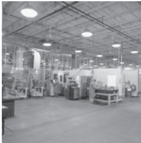
The Mazak Mazatrol Flexible Machining System (FMS). The FMS cell features three horizontal mill machining centers, each served with a 120 tool capacity automatic tool changer. A vertical pallet stacker crane robot delivers pallets to the machining centers. Set-up time is reduced to zero. Raw casting to finished, inspected parts all completed within the FMS cell, making very short lead times possible.
