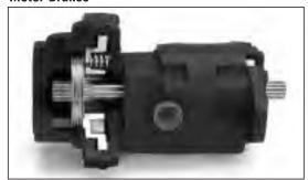
All Rol-Seal® motors can be equipped with a rearmounted, normally on, wet friction disc type brakes. They will prevent creep under high static loads which might result from system leakage. They also should be used where positive locking of the motor shaft is required.
